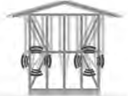
耐震工法+MER System
